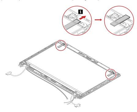
2. Turn over the LCD panel and then detach the LCD cable from the LCD panel as shown.
