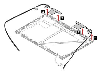
Attention: As you route the cables, ensure that they are not subject to any tension. Tension could cause the cables to be damaged by the cable guides, or a wire to be broken.
