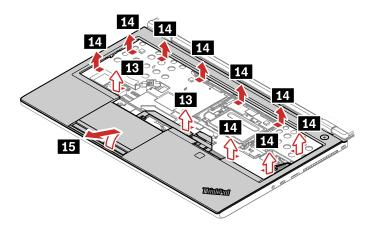
When installing: Ensure that all the latches are well assembled and there is no abnormal gap.
