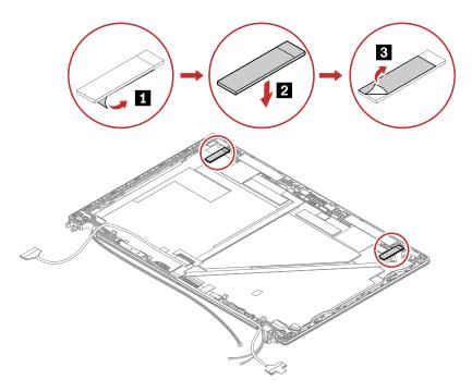
2. Attach the LCD cable to the LCD panel as shown. Turn over the LCD panel to secure the LCD panel with tapes.
