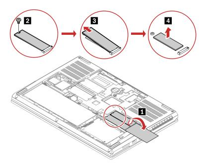
When installing: If your computer is installed with only one M.2 solid-state drive, ensure that the M.2 solidstate drive is installed into slot 0.
