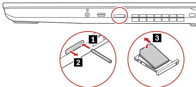
After you finish the servicing, ensure that you install the nano-SIM card back into the slot firmly.
