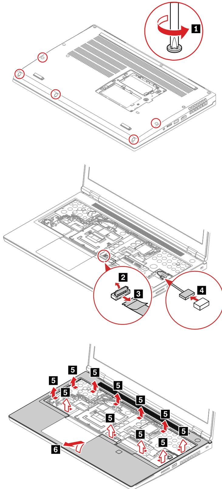
**When installing:** Ensure that all the latches are well assembled and there is no abnormal gap.
