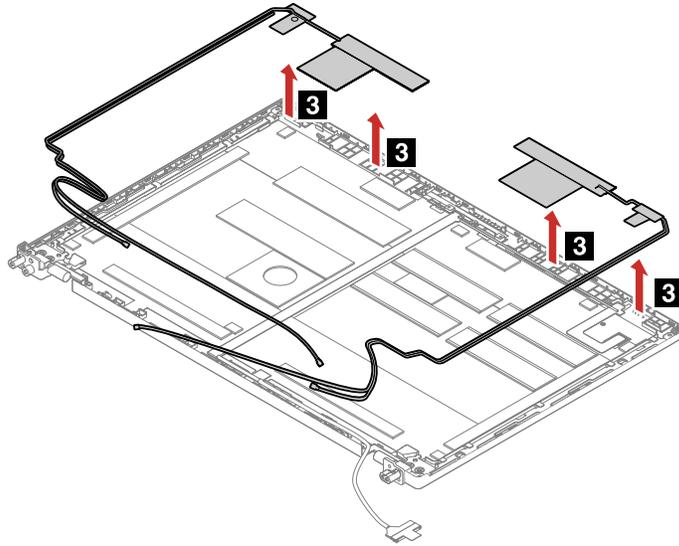
**Attention:** As you route the cables, ensure that they are not subject to any tension. Tension could cause the cables to be damaged by the cable guides, or a wire to be broken.
