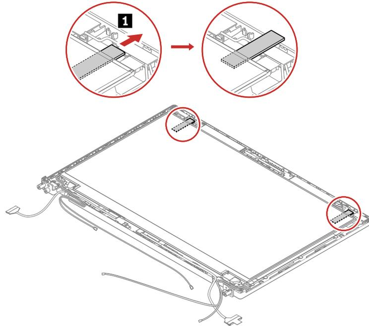
2. Turn over the LCD panel and then detach the LCD cable from the LCD panel as shown.
