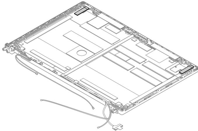
2. Attach the LCD cable to the LCD panel as shown. Turn over the LCD panel to secure the LCD panel with tapes.
