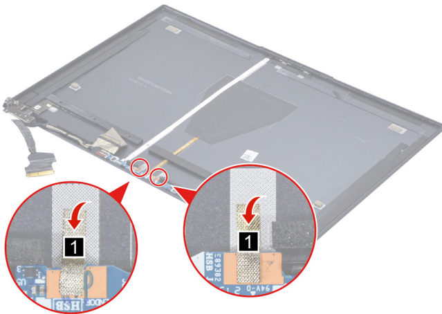
Figure 38. Remove the two pieces of microphone board conductive tape
