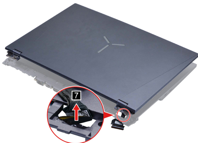
Figure 32. Take out the EDP cable and then remove the LCD module
