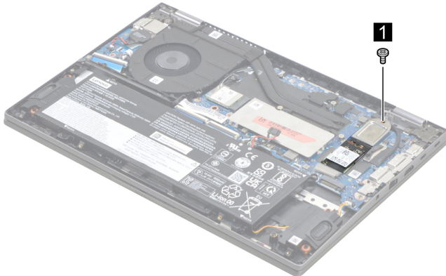
Figure 6. Remove one screw
