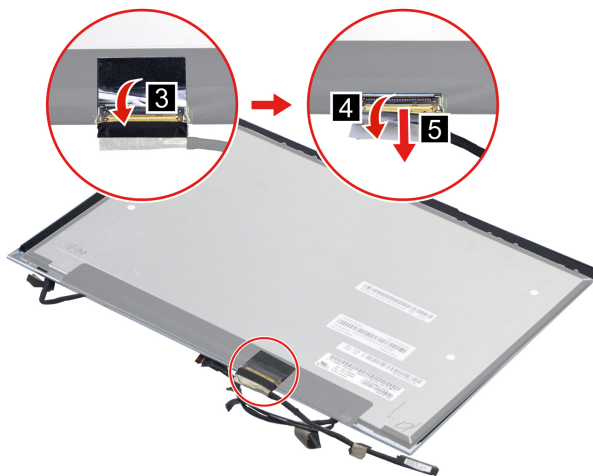
Figure 32. Remove the EDP cable
