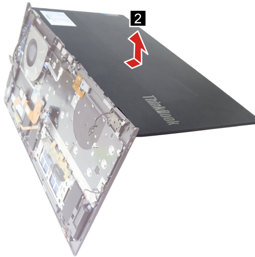
Figure 33. Rotate the LCD module and remove the LCD module
