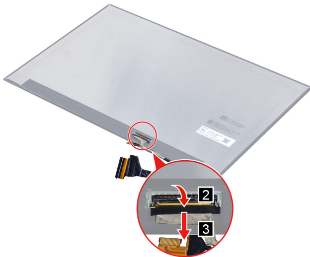
Figure 61. Remove the EDP cable
