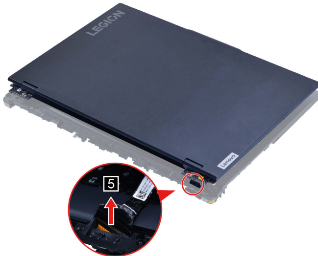
Figure 50. Take out the EDP cable and remove the LCD module
