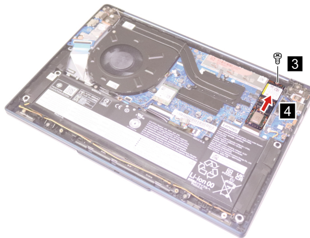
Figure 12. Remove the 2280 solid-state drive
