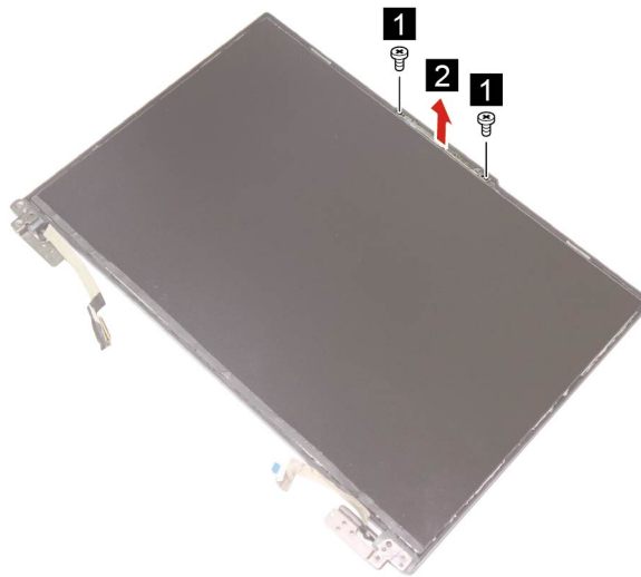
Figure 32. Remove two screws and remove the camera bracket
