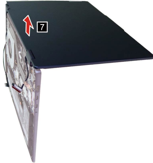
Figure 51. Rotate and remove the LCD module
