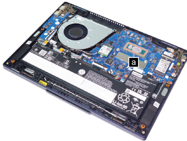
Figure 3. Area on the system board where thermal interface materials is applied
