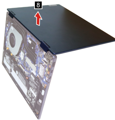
Figure 48. Rotate and remove the LCD module
