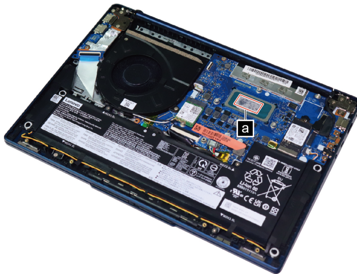
Figure 4. Area on the system board where thermal interface materials are applied
