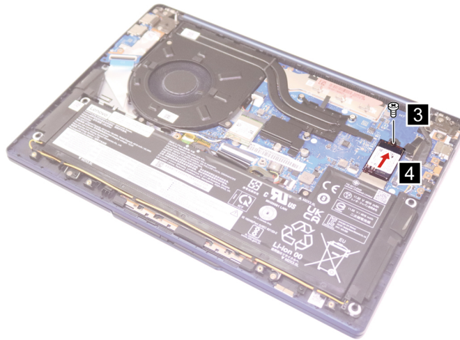
Figure 12. Remove one screw and remove the solid-state drive
