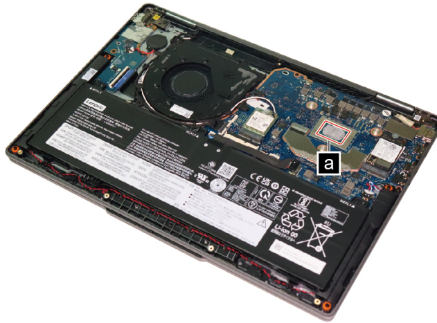
Figure 3. Area on the system board where thermal interface materials are applied
