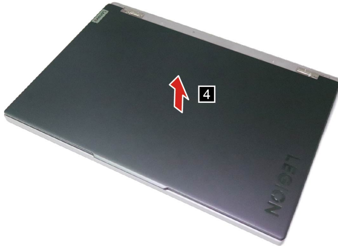
Figure 30. Remove the LCD unit
