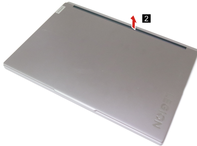
Figure 26. Remove the hinge cap
