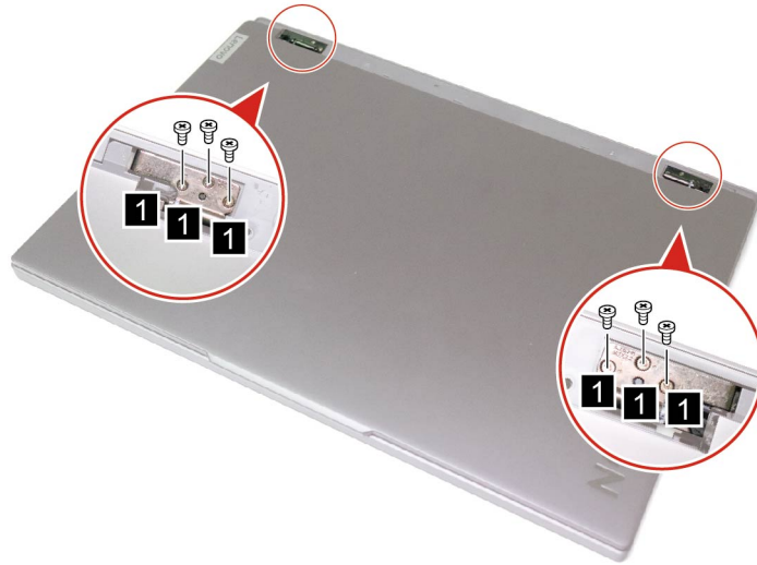
Figure 28. Remove six screws
