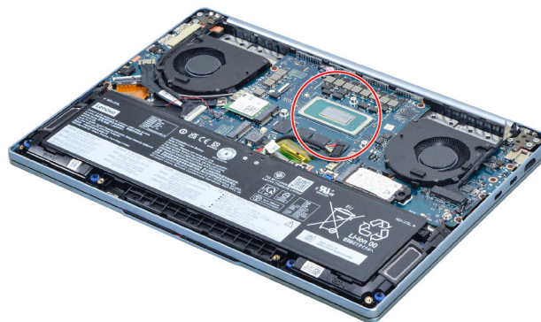
Figure 6. Areas on the system board where thermal interface materials are applied
