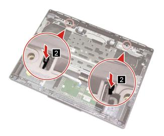
Figure 42. Release the hooks
