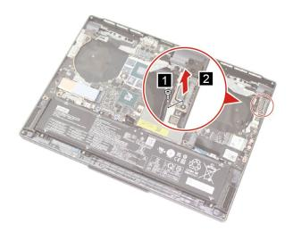
Figure 36. Remove one screw and the USB-A bracket
