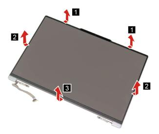
Figure 46. Lift and remove the LCD bezel
