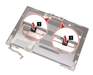
Figure 52. Remove the microphone rubbers
