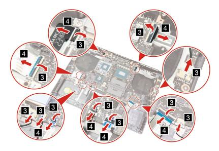
Figure 38. Disconnect all the cables from the system board
