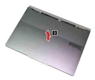
Figure 45. Remove the LCD module
