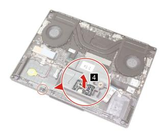
Figure 18. Remove the Hall sensor board
