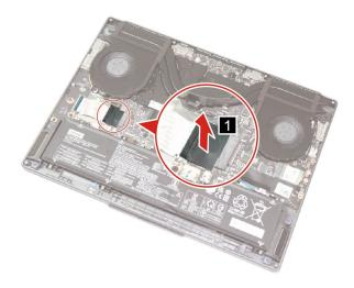
Figure 31. Peel off the I/O board connector mylar
