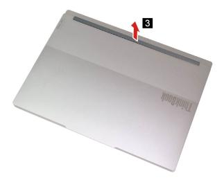
Figure 43. Remove the hinge cap
