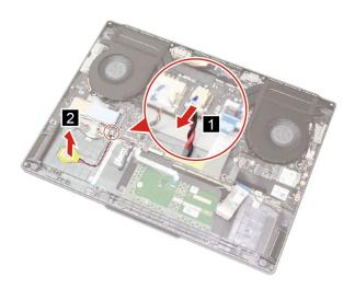
Figure 19. Remove the coin-cell battery
