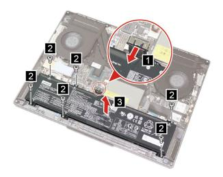
Figure 6. Remove six screws and the battery pack
