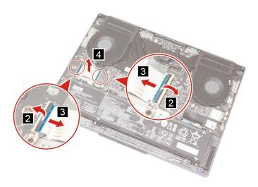
Figure 32. Disconnect and remove the I/O board cable
