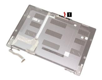
Figure 51. Remove the camera shutter
