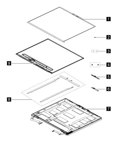
Figure 2. LCD exploded view
