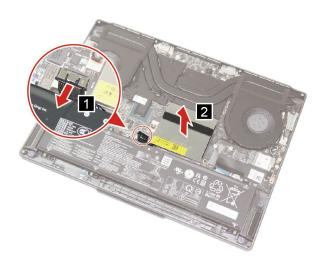
Figure 7. Remove the memory shielding
