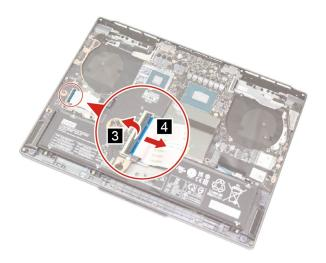
Figure 34. Disconnect the I/O board cable
