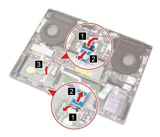
Figure 17. Remove the Hall sensor board cable
