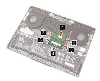
Figure 8. Remove the memory modules
