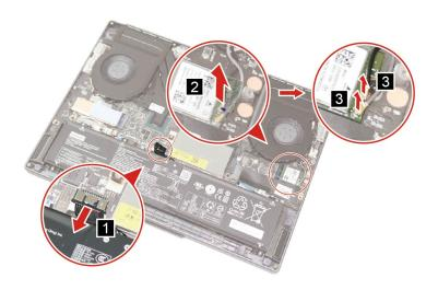
Figure 23. Disconnect the battery pack cable, peel off the Wi-Fi card mylar and disconnect the Wi-Fi antennas
