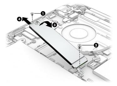
4. When installing an SSD, be sure a thermal pad is installed on the bottom of the drive bracket as shown in the following illustration.
