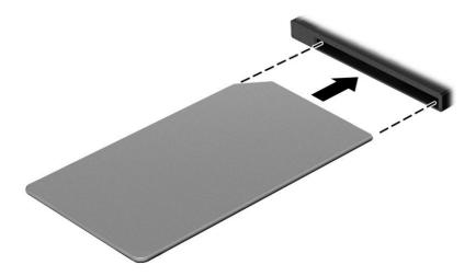
To remove the SIM card, press in gently on the card to disengage the SIM lock, and then remove it from the slot.
