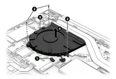
To install the fan, reverse this procedure.
