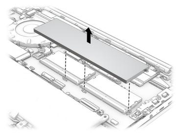
2. Spread the two retention clips outward (1) until the memory module tilts up at a 45° angle, and then remove the module (2). Use the same procedure to remove all memory modules.
