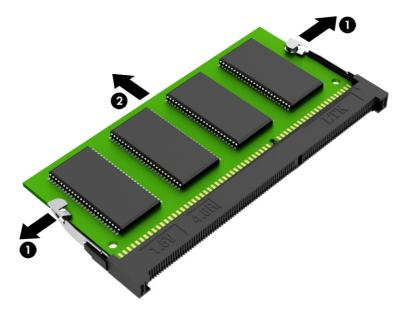
To install a memory module, reverse the removal procedures.
