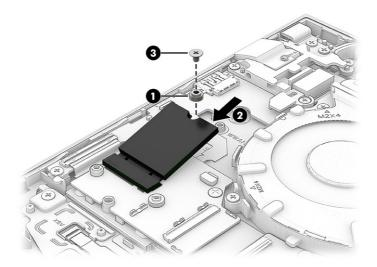
To install the solid-state drive, reverse the removal procedures.
