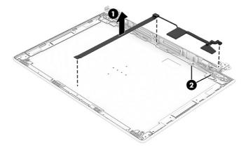
17. To remove the wireless antennas and cables:
