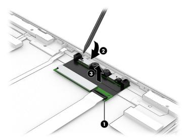
b. IR cameras use different black protective tape depending on the panel. When installing a new IR camera, be sure to add new tape that matches the shape of the tape on the old camera.
