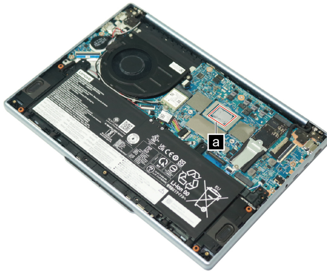
Figure 4. Areas on the system board where thermal interface materials are applied
