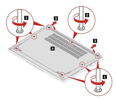
Step 2. Install the base cover assembly as shown below.
