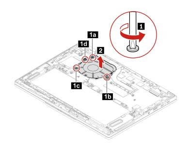
Step 2. Install the thermal fan assembly in reverse order.
