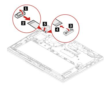
Step 3. Install the power button with fingerprint reader and fingerprint reader cable in reverse order.
