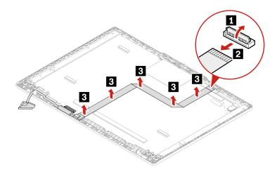
Step 2. Install the LCD cable in reverse order.
