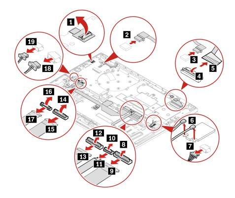
Remove the system board as shown below.
