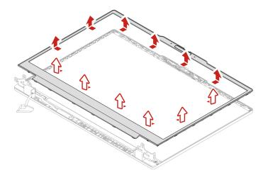
Step 2. Install the LCD bezel in reverse order. When installing, ensure that all the latches are attached firmly.
