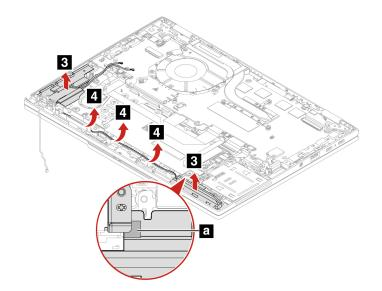
Step 3. Install the wireless WAN antenna assembly in reverse order.
