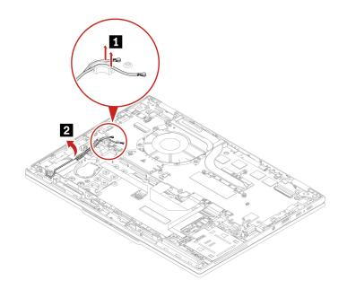
Step 2. Remove the wireless WAN antenna assembly as shown below. (When installing, ensure that the gasket on copper-foil is under the trackpad bracket.)
