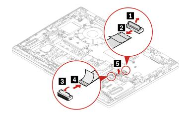
Step 2. When installing: Ensure that the connectors are attached firmly.
