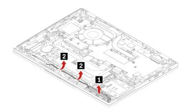
Step 2. Remove the Wireless LAN antenna kits as shown below.
