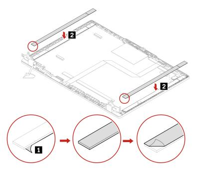
Step 2. Attach the LCD cable to the LCD panel as shown. Turn over the LCD panel to secure the LCD panel with tapes.
