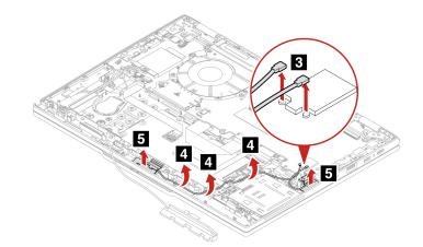
Step 3. Install the wireless WAN antenna assembly in reverse order.
