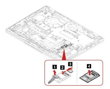
Step 2. When installing: Ensure that the connectors are attached firmly.
