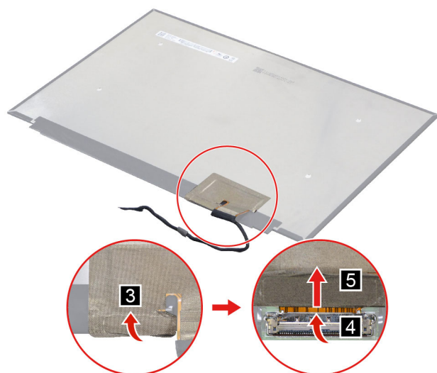
Figure 43. Remove the EDP cable
