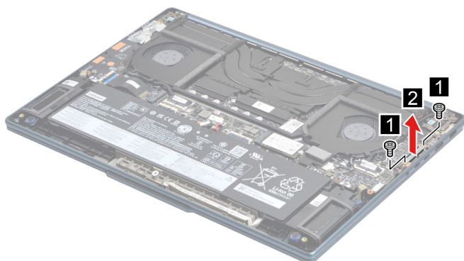
Figure 19. Remove the Type-C bracket
