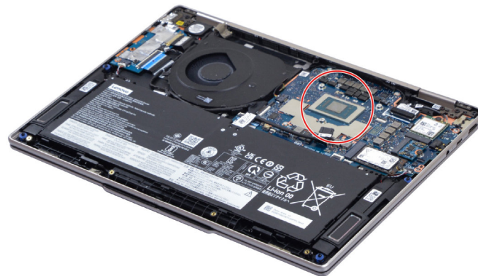
Figure 40. Areas on the system board where thermal interface materials are applied (AMD models)
