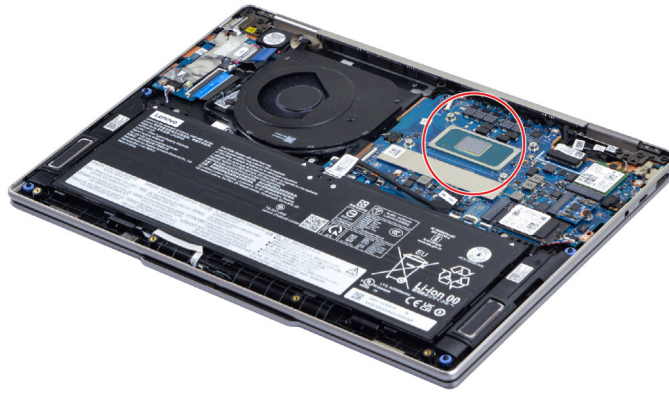
Figure 41. Areas on the system board where thermal interface materials are applied (Intel models)
