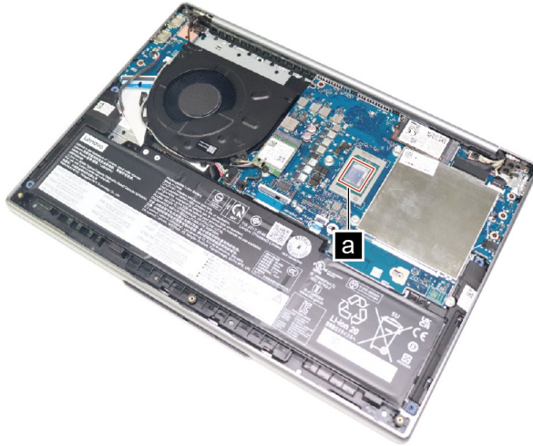
Figure 16. Areas on the system board where thermal interface materials are applied (for AMD models)
