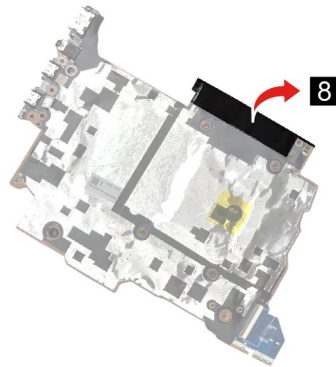
Figure 86. Peel off the MB acetate tape covering the PMIC board and the PMIC cable
