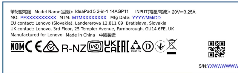
Figure 98. Artworks for the laser etched label used in worldwide countries or regions
