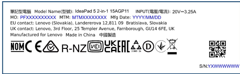
Figure 122. Artworks for the laser etched label used in worldwide countries and regions
