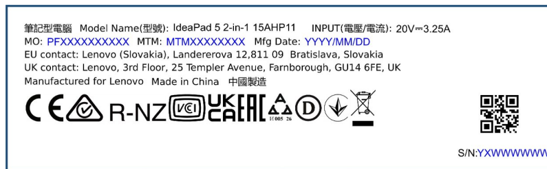
Figure 134. Artworks for the laser etched label used in worldwide countries and regions
